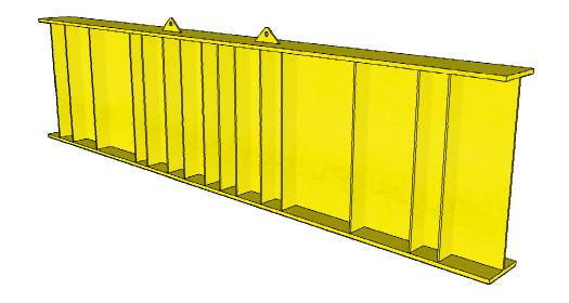
An 8 m high-capacity loading beam used in modular configurations of reaction systems. It is composed of high strength steel and contains lateral stiffeners across its span and integrated lifting eyes.
