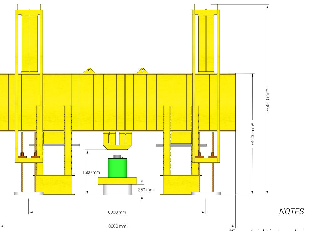
\*Frame height is dependent on pile cap elevation; frame adjusted to accommodate using trestles
