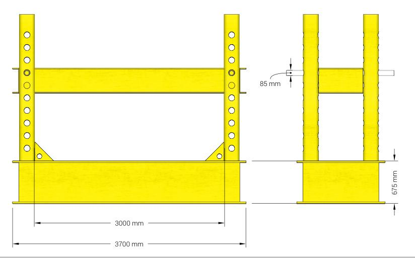
The trestles are used in pairs to support the beams and tension elements above the test pile. The main platform can be adjusted in height to suit the elevation of the test pile cap using removable, high strength pins. The trestle is composed of high strength steel and includes integrated lifting eyes.
