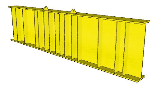
An 8 m high-capacity loading beam used in modular configurations of reaction systems. It is composed of high strength steel and contains lateral stiffeners across its span and integrated lifting eyes.
