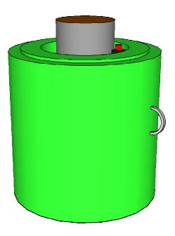
The hydraulic actuator is used to apply the load force to the foundation element. It has a maximum operating pressure of 690 bar with an over-pressure rating of 1035 bar. It has a maximum capacity of 15 MN and hydraulic stroke of 250 mm. It is fitted with two swivel lifting eyes for easy handling. For added safety and stability it has a recessed rod-end cavity to house the load cell.
