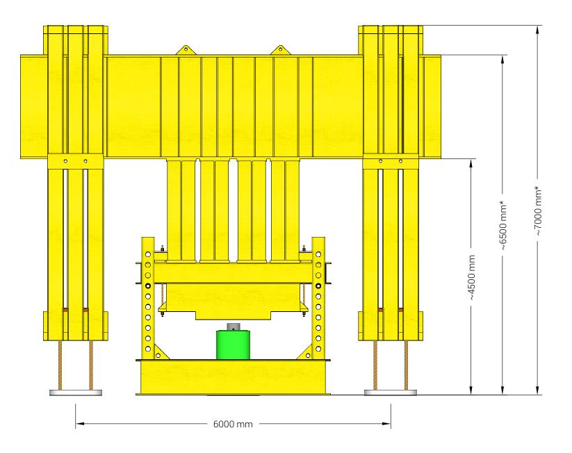
\*Frame height is dependent on pile cap elevation; frame adjusted to accommodate using trestles
