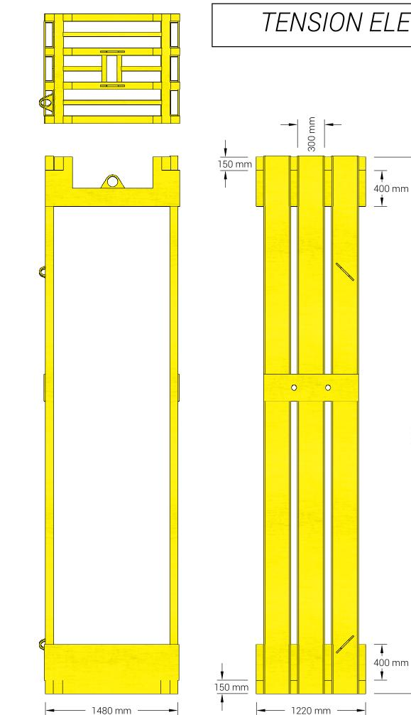
The tension element hangs from the secondary beams and provides a restraint lower than the load application providing increased stability and reducing the need for working at height. It is composed of high strength steel and at each end comprises a loading plate with integrated loading beams. Each end is connected by 6 no. 300 mm channels. A mid-span brace is attached on both sides and lifting eyes are integrated on two faces to allow both horizontal transport and vertical operation.
