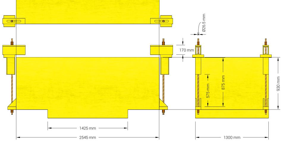
The saddle is positioned above the test piles and is used to apply the load evenly in to the primary beams. It is held in place by four moveable clamps which attach to the bottom flange of the outermost primary beams.
