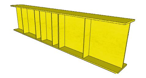
A 4 m high-capacity loading beam used in modular configurations of reaction systems. It is composed of high strength steel and contains lateral stiffeners across its span and integrated lifting eyes.
